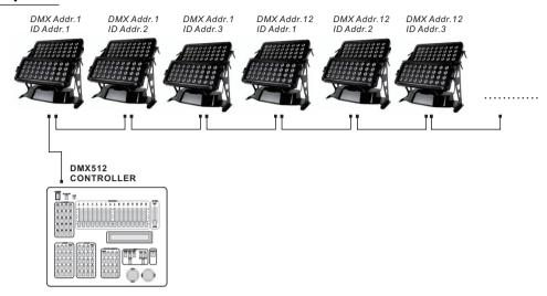
The figure above shows a simple DMX layout which has used three units at each DMX address. The three units have different ID addresses which allows the user to collectively control the whole group of units at that DMX address by setting CH11 to 0, or to control each unit independently by first selecting the DMX address and then by using CH11 to locate the target ID address.
